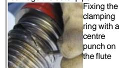
Fixing the clamping ring with a centre punch on the flute
