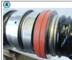
Mask a beginning of a nipple with a thin layer of duct tape.
